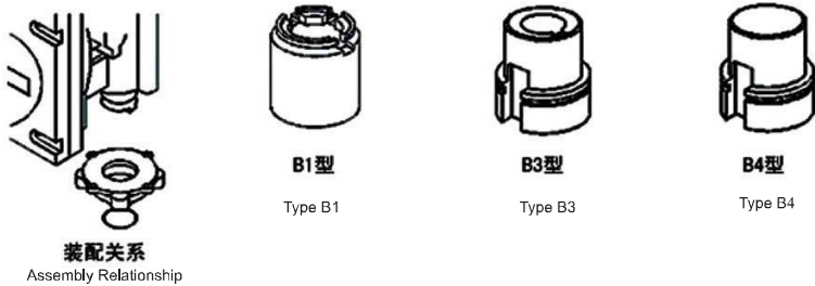
Picture 5-2 Sketch Map of Connection Form of Split-type Mounting Base with Non-thrust Drive Sleeve of EMS30-EMS550 Actuators
