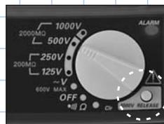
Protection against inadvertent setting of rotary switch to 1000 V rating
