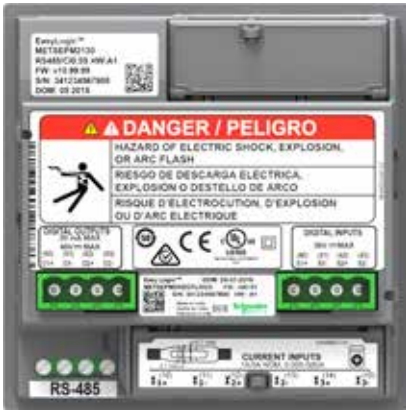
Rear of PM2000 with I/O module
