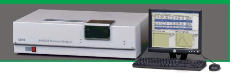
**Instrument Range** @ **100 mg** Mercury: 0.5 ppb to 5 ppm (0.05 to 500 ng absolute)
