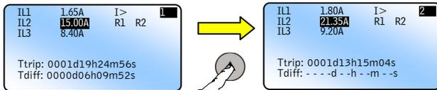
The example on the left shows the problem on phase L2 on both trip events. The difference between the first recorded trip and second was **6h 09m and 52s**.
