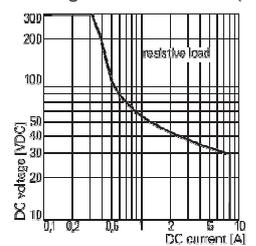
Max. DC Load Breaking Capacity
