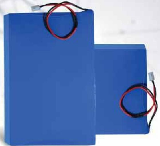
Lithium-iron-phosphate (LiFePO<sub>4</sub> or LFP) is the safest of the mainstream li-ion battery types. The nominal voltage of a LFP cell is 3,2V (lead-acid: 2V/cell). A 12,8V LFP battery therefore consists of 4 cells connected in series; and a 25,6V battery consists of 8 cells connected in series.
