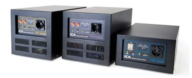
The UPS inverter works only when the AC input voltage low or loss. When the AC input voltage in normal condition, UPS will stabilize and filter the AC input voltage and supply a clean and stable AC voltage to the UPS output and charge the battery. When the AC input voltage is low or loss, inverter will replace it and supply a stable AC voltage within a very short transfer time.
