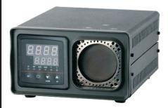
BX-500 Portable IR Calibrators are used for calibrating Infrared Thermometers. Whether you're using in-line or handheld infrared pyrometers, you need a high performance calibration standard to verify accuracy. Portable IR Calibrator provides a stable black body target for calibrating non-contact IR thermometers up to 500°C.
