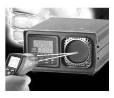
For even higher precision, a contact calibration well is located directly behind the blackbody surface. Using an optional digital RTD Thermometer and calibrated secondary probe, accuracies of  $\pm\,0.1^{\circ}\text{C}$  can be achieved.
