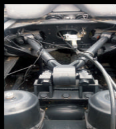
Double Circuit Full Air Brake with brake chamber on save position
