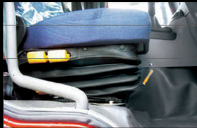
Seat with Air suspension system for driver comfort and position adjustment
