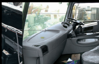
Spacious cabin and Steer System with P/S and Tilt steering wheel
