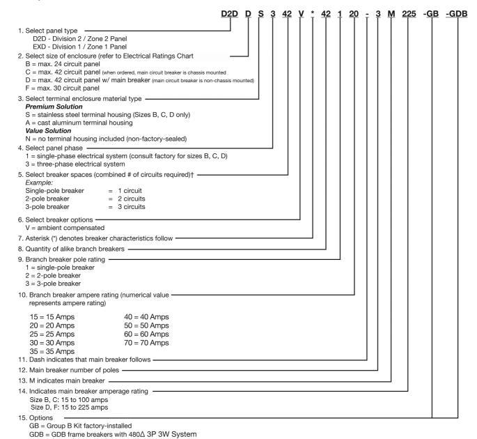
† Group B and IIB + H2 is standard on all PowerPlus panels, but requires special brackets to be installed on breakers to ensure long-term operability of circuit breakers. To order with brackets installed at factory, add suffix -GB. For field installable kit, order EXD-GB-KIT for sizes B, C and D separately. ‡ NEMA 4X rating is available when ordered with suffix S752 or S753.
