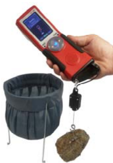
Density Measurement: Sample in Air
