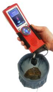
Density Measurement: Sample Submerged in Water
