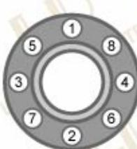
When installing flanges, it is critical that bolts be equally tightened in sequence which diametrically opposed to each other.
