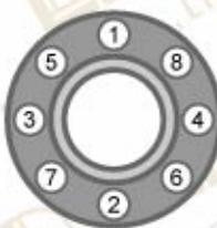
When installing flanges, it is critical that bolts be equally tightened in sequence which diametrically opposed to each other.
