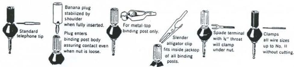
Figure 2-3. Methods of connection to binding-post terminals.
