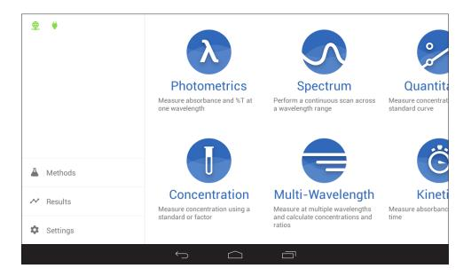
These spectrophotometers are controlled solely through the touchscreen interface of the equipment and follow a basic Android user interface. If the number of options available in a menu exceeds the number that can be displayed on the screen, swipe to the left to view the other modes.
