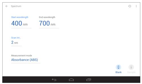
The start and end wavelengths must be different. If the same value is entered an error message will be displayed.
