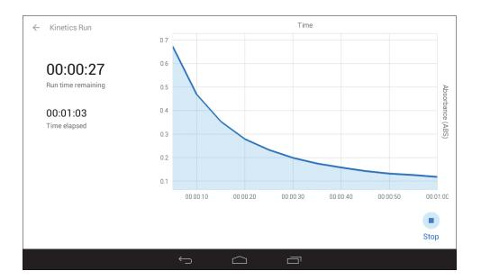
Once the measurement time is complete the full kinetics run will be shown on the screen. To run the kinetics experiment again using the same method parameters touch **RUN AGAIN**. Subsequent samples can be measured in the same way. If the wavelength is adjusted between sample measurements then the instrument must be calibrated again before more samples can be measured.
