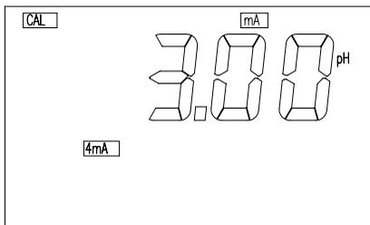
This screen will let the user change the 4 mA value. The user can use [▲], [▼], [▶] or [OK] keys to input new 4mA value. This value is used for scaling the 4-20mA **ANALOG OUTPUT**. (For detailed explanation see chapter **VI. 4-20 mA OUTPUT**.)
