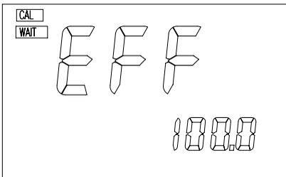
This screen will display the efficiency of the pH electrode from its last calibration. This screen is for user information only and will automatically change to the 4mA setting after 4 seconds.
