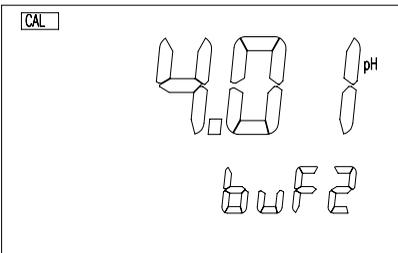
This screen selects the buffer for slope calibration. The user can select "1.68pH", "4.00pH", "4.01pH", "9.18pH", "10.01pH" or "12.46pH". Press the [ $\blacktriangle$ ] or [ $\blacktriangledown$ ] keys to select the buffer then the [OK] key to save your selection.
