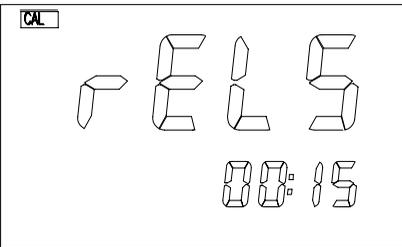
This screen set the ON TIME delay in **MINUTES:SECONDS** for the **RELAY 5**. The user can use [▲], [▼], [▶] or [OK] keys to input the new ON time. You can only turn-ON the WASH relay if the unit is UNLOCKED.
