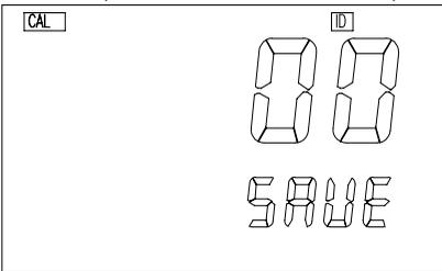
This screen selects the unique ID/ address for the unit. Your RS485 communication program must also use this same ID to communicate with this unit. The user can use [▲], [▼], [▶] or [OK] keys to input the new ID/ address.
