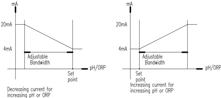
The above figure shows the relationship between Reading,  $U_{4mA}$  &  $U_{20mA}$ .
