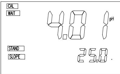
After finishing the Buffer I calibration the unit will move to this screen. The initial display will be the chosen buffer for **pH BUFFER II SELECT**. The “**SLOPE**” annunciator will blink indicating that the unit is waiting for the user to continue the calibration.
