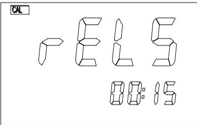
This screen selects the ON TIME delay in MINUTES:SECONDS for the RELAY 5. The user can use [▲], [▼], [▶] or [OK] keys to input the new ON time. You can only turn-ON the WASH relay if the unit is UNLOCKED.
