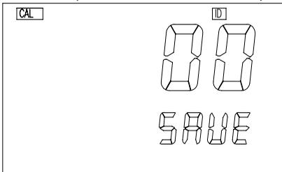
This screen selects the unique ID/address for the unit. Your RS485 communication program must also use this same ID/ address to communicate with this unit.
