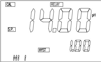
This screen is essentially the same for the four relays. Take note of the blinking character as there are 3 values to input for each relay. The user can use [▲], [▼], [▶] or [OK] keys to input the **SET-POINT** then the **HYSTERISIS** and finally the
