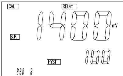
This screen is essentially the same for the four relays. Take note of the blinking character as there are 3 values to input for each relay. The user can use [ $\blacktriangle$ ], [ $\blacktriangledown$ ], [ $\blacktriangleright$ ] or [OK] keys to input the SET-POINT first then the HYSTERISIS and finally the RELAY ACTION. (See V. CONTROLLING THE RELAYS.)
