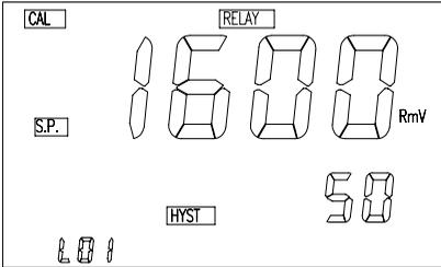
This screen is essentially the same for the four relays. Take note of the blinking character as there are 3 values to input for each relay. The user has to input the SET-POINT first then the HYSTERISIS and finally the RELAY ACTION.
