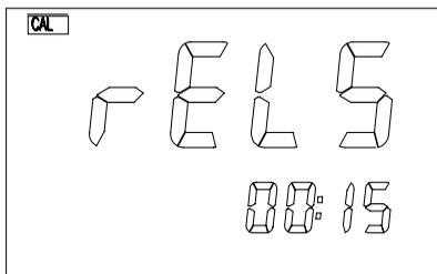
This screen selects the ON TIME delay in MINUTES:SECONDS for the RELAY 5. The user can use [ $\blacktriangle$ ], [ $\blacktriangledown$ ], [ $\blacktriangleright$ ] or [OK] keys to input the
