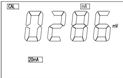
This screen will let the user change the 20 mA value. The user can use [ $\blacktriangle$ ], [ $\blacktriangledown$ ], [ $\blacktriangleright$ ] or [OK] keys to input new 20mA value. This value is used for scaling the 4-20mA ANALOG OUTPUT. (For detailed explanation see chapter VI. 4-20 mA OUTPUT.)
