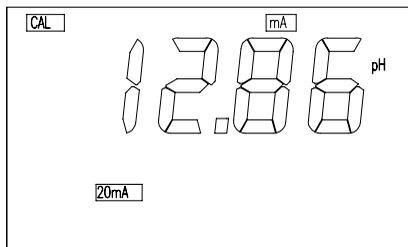
This screen will let the user change the 20 mA value. The user can use [▲], [▼], [▶] or [OK] keys to input new 20mA value. This value is used for scaling the 4-20mA **ANALOG**
