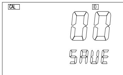
This screen selects the unique ID/address for the unit. Your RS485 communication program must also use this same ID/ address to communicate with this unit. The user can use [▲], [▼], [▶] or [OK] keys to input the new ID/address.
