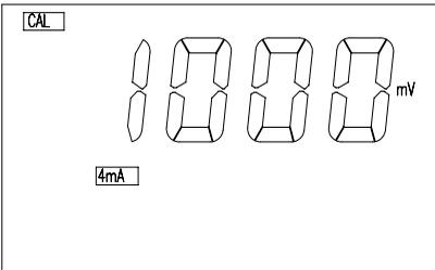
This screen will let the user change the 4 mA value. The user can use [ $\blacktriangle$ ], [ $\blacktriangledown$ ], [ $\blacktriangleright$ ] or [OK] keys to input new 4mA value. This value is used for scaling the 4-20mA ANALOG OUTPUT. (For detailed explanation see chapter VI. 4-20 mA OUTPUT.)
