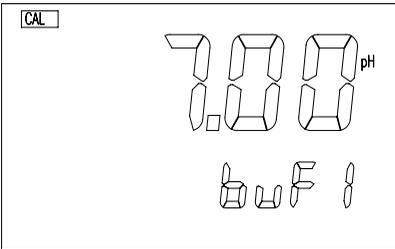
This screen selects the buffer for standardization calibration. The user can select "7.00pH" or "6.86pH". Press [ $\blacktriangle$ ] or [ $\blacktriangledown$ ] keys to select the buffer then the [OK] key to save your selection.
