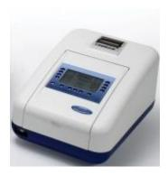
This highly anticipated spectrophotometer incorporates Jenway's Microvolume accessory with the dedicated life science measurement modes of the Genova Plus - along with those of a standard spectrophotometer. This makes the Genova Nano Jenway's first 3 in 1 spectrophotometer.
