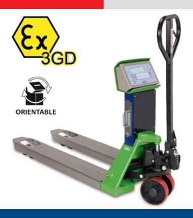
Pallet truck scales, with built-in electronic weighing, suitable for harsh working conditions and dangerous areas classified as hazardous (ZONE 2, 22) in accordance with Ex II 3G IIC T6 Gc X and Ex II 3D IIIC T115C° Dc X protection. The Atex certified four load cell weight detection guarantees the best accuracy in all work conditions. Manufactured, calibrated and adjusted in Italy by Dini Argeo, using certified sample masses.
