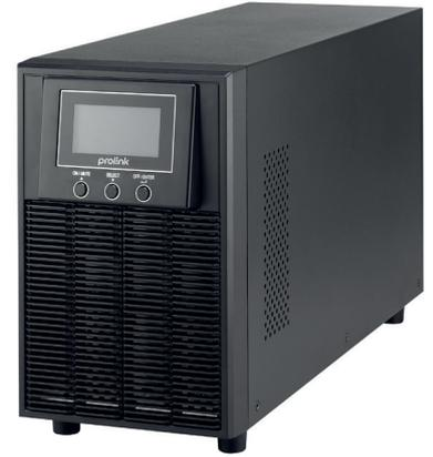
ProLink **Master II Series (1P/1P) Tower Type** is a single-phase UPS system that employs a true online double-conversion technology. UPS system is designed to deliver clean and high quality electrical power to fully protect critical devices such as sensitive networks, small computer centres, servers, medical equipment, telecom applications as well as industrial applications. High input power factor correction in the system improves the efficiency and reduces overall losses.
