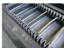
Side Wall Belt Conveyor
